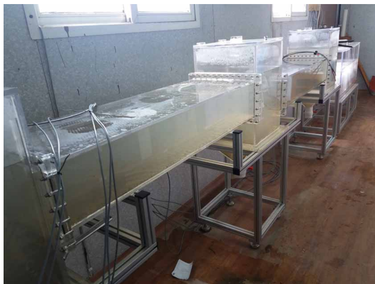
Figure 7 | Pilot scale treatment system filled with first flush storm water for experiment at the study site.
